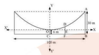
Here, AB and OC are the longest and the shortest wires, respectively, attached to the cable. DF is the supporting wire attached to the roadway, 18 m from the middle.
