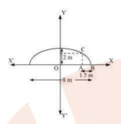
The equation of the semi-ellipse will be of the form  $\frac{x^2}{a^2} + \frac{y^2}{b^2} = 1$  y  $\geq 0$ , where a is the semi-
